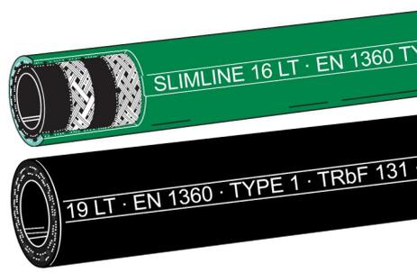
"CONTI" quality petrol pump hoses for gasoline and diesel. Can be gauged for electric dispensing pumps, see explanation overleaf. Flexible down to - 30° C / - 22° F (LT-type down to - 40° C / - 40° F). Correspond to TRbF 131/2 and EN 1360.
